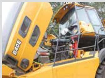
The cab can be tilted in minutes without special tools, for convenient service access to drivetrain components.
