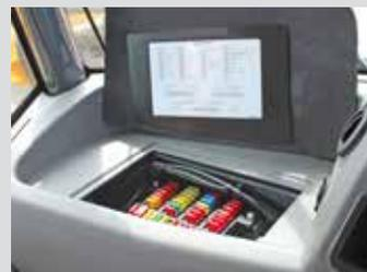
An in-cab load centre simplifies fuse replacement. Fewer relays, connectors and harnesses mean higher reliability.
