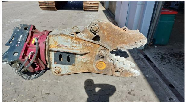
**Demarec, Betonpulverisierer DLP16, OQ65**
