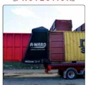
To transfer the load, the truck reverses and the shipping container encapsulates the loading chamber until it reaches the end. As the truck drives forward, pulling the slide with it, the load is held inside. This system ensures that you achieve virtually no container damage.
