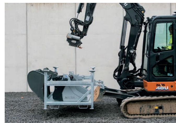
Optimised installation height thanks to the recessed adapter frame, resulting in greater digging force and less machine stress.
