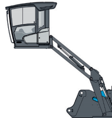
Cab system vertically adjustable and horizontally adjustable
