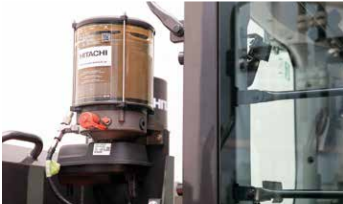
Optional auto-greasing system saves time.
