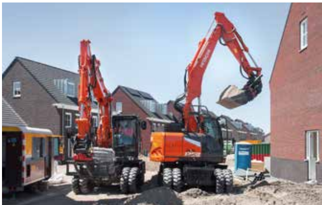
The ZX135W-7 turns within a radius of 3.5 metres (1,740mm to the rear and 1,750mm to the front).
