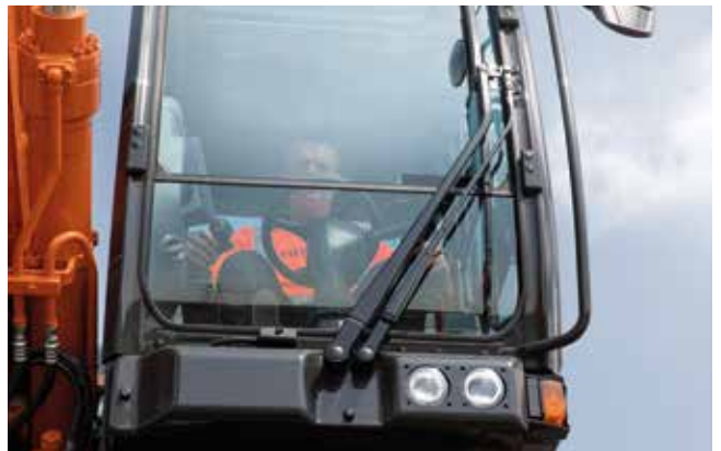
Wider wiper design provides greater visibility.
